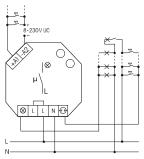
4-wire circuit with attic lighting, resettable
