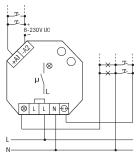
3-wire circuit, resettable
