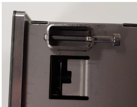
Mounting bracket engaged on PQI-DE
